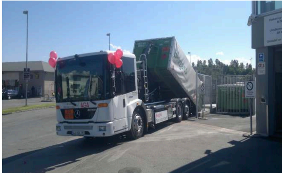
Figure 5. Hook-loaded biogas transport and storage module by AGA (a predecessor company of Gasum) (AGA, 2012).
