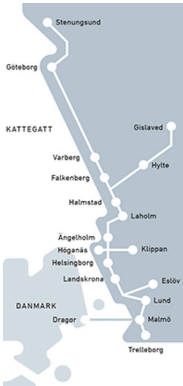
Figure 7. The Swedish methane gas grid (Swedegas 2020).
