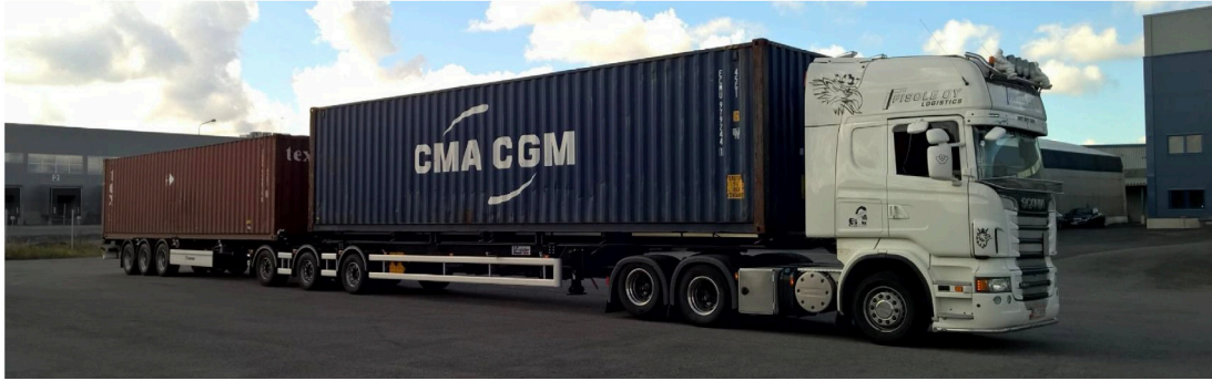
Figure 4. B-link (B-train) with 2x40 ft containers in Finland 16 .
