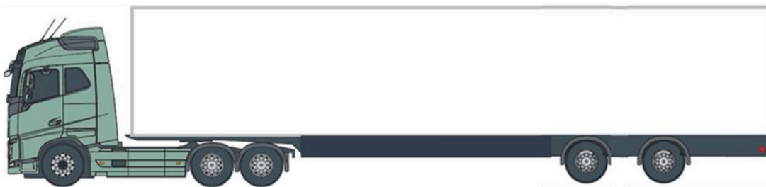
Figure 5. An illustration of 5 axles truck-trailer with a maximum total weight of 44 tonnes 17 .
