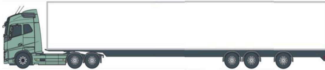
Figure 6. 6-axis articulated vehicle (max. 17.5 m), modified from 19 .
