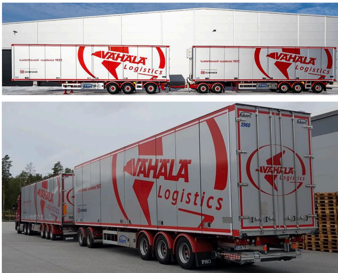
Figure 3. A-double 2x13.6 trailers in Finland 15 .
