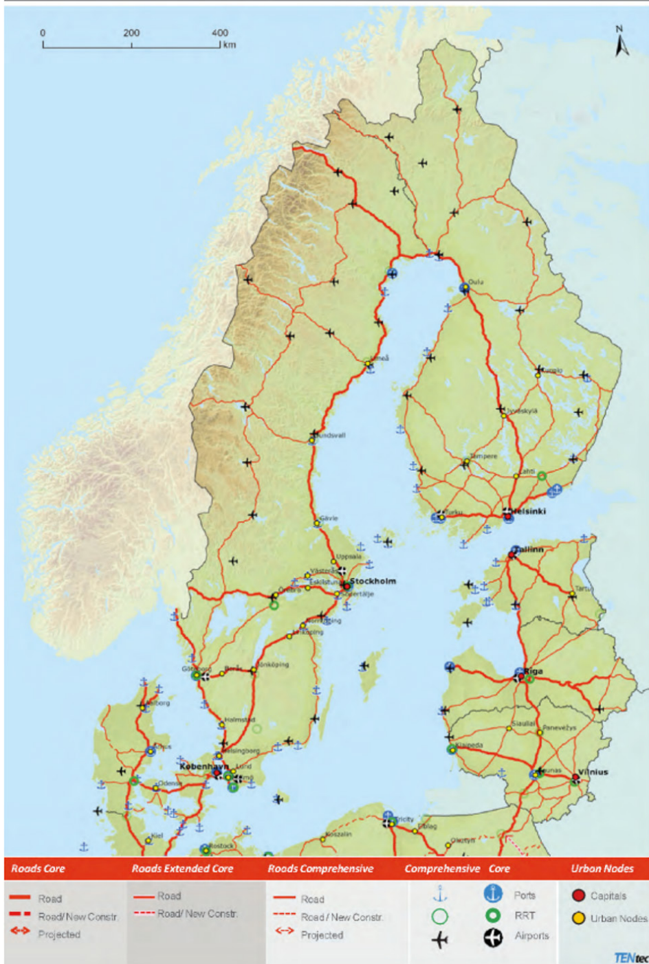
Figure 12: Core, Extended Core and Comprehensive Network Roads, ports, rail-road terminals and airports 3 .
